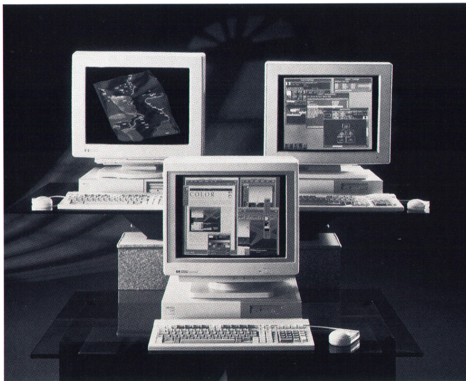
Fig. 1. The HP 9000 Models 705 (right) and 710 (left and center) workstations are 35-MHz and 50-MHz entry-level members of the HP 9000 Series 700 family.
